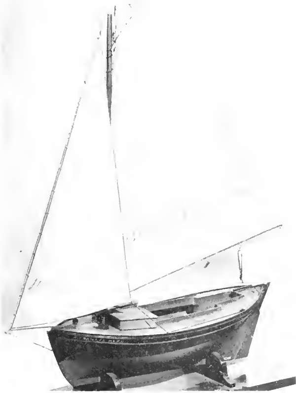
QUODDY BOAT Yankee Hero , 1889. Rigged model USNM 76266. An average size boat of her type, she was built to carry sardines from the weirs to the canneries. The builder's half-model of this boat is USNM 76293. (Smithsonian photo 44065 g.)
